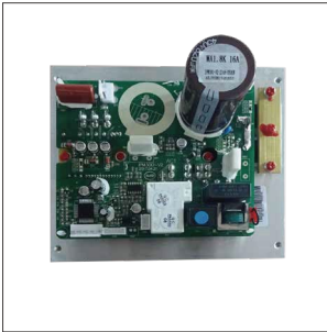
④ Inverter board
